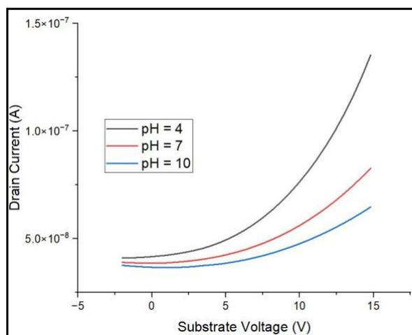
**Figure 3.** ISFET transfer characteristics with different pH values.
