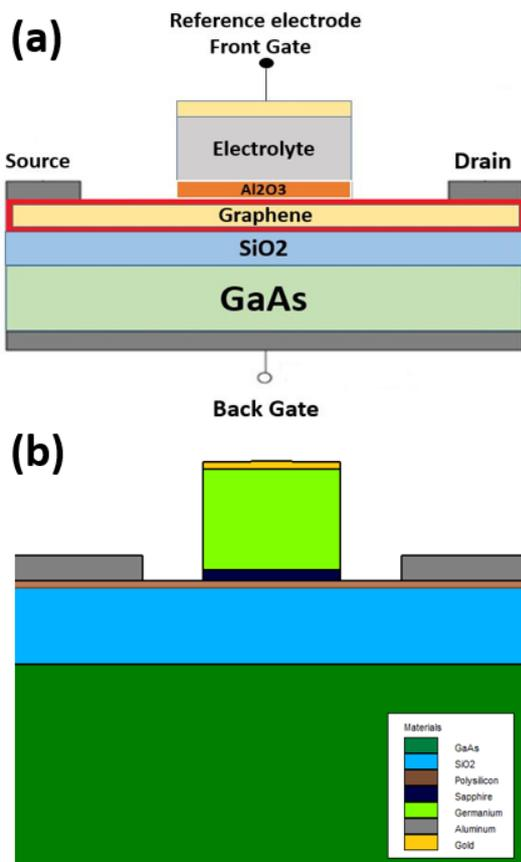
**Figure 1.** (a) Block diagram and (b) constructed structure of graphene based ISFET in Silvaco.
