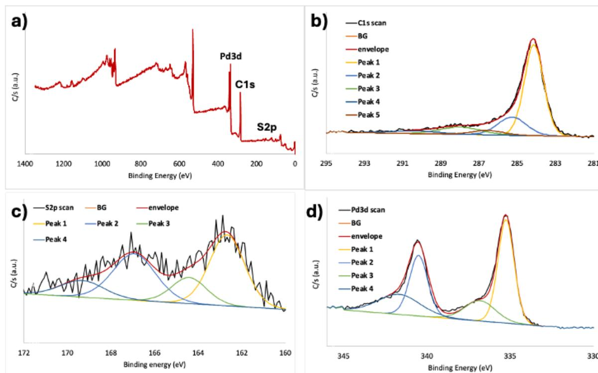
**Figure 2.** XPS Results of Pd-SO<sub>3</sub>H/CNO; a) general XPS survey, b) C1s, c) S2p, and d) Pd3d peaks.
