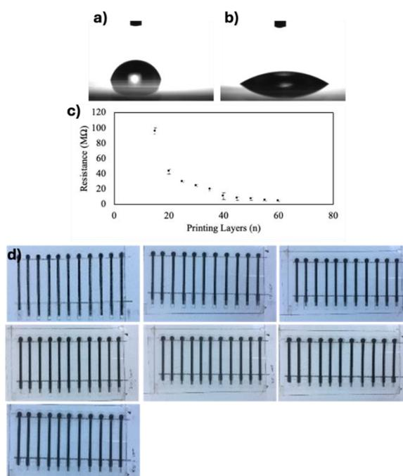
**Figure 3.** Contact angle measurement results obtained from a) untreated PET and b) plasma-cleaned PET, c) the effect of the number of printing passes on the resistance of the prints, and d) digital images of the prints taken at different printing passes.
