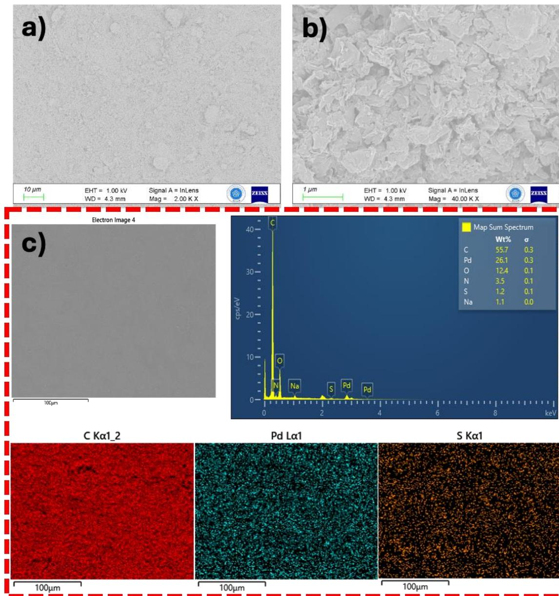
**Figure 4.** a-b) SEM images of the printed electrodes at different magnifications, c) EDS mapping results.
