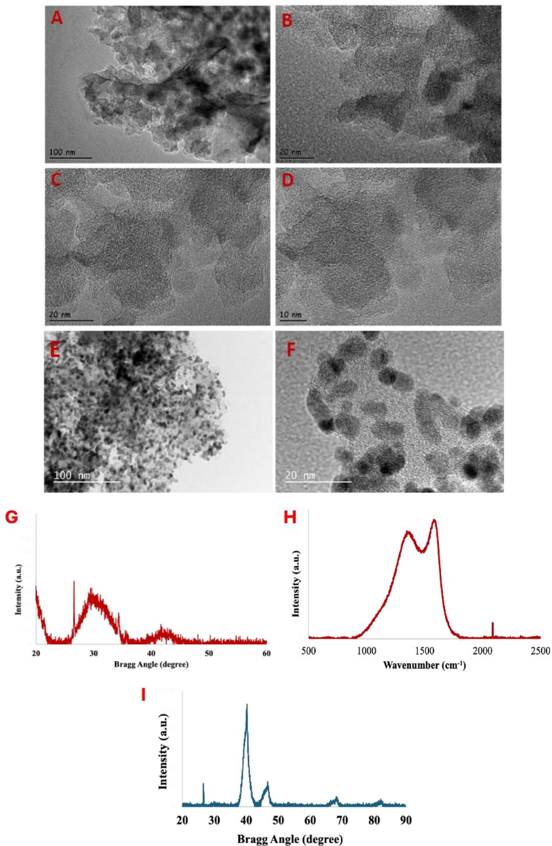
**Figure 1.** Physical characterizations of CNO: a-d) TEM images of CNO, e-f) TEM images of Pd-SO<sub>3</sub>H/CNO, g) XRD and h) Raman spectrum of CNO, and i) XRD pattern of Pd-SO<sub>3</sub>H/CNO.
