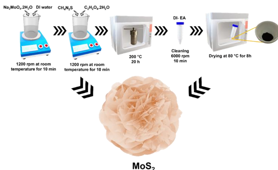
Figure 8. Schematic illustration of the synthesis procedures of flower-like MoS 2 .
